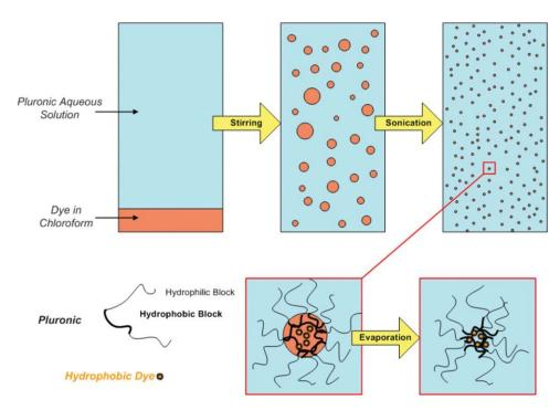
Fig. 2 Schematic representation of the Pluronic micelles synthesis (see text for details).
