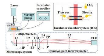
**Fig. 1** Experimental setup of QPM for the examination of a live cell. Inset is incubator chamber system.
