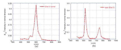
**Fig. 3** (a) Simulated transmitted electric field intensity for a single OLED. (b) Simulated transmitted field intensity for a tandem OLED with an intermediate Ag thickness of x = 10 nm.
