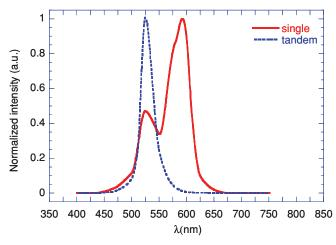
Fig. 4 Simulated emission intensity for microcavity single unit and tandem OLEDs.
