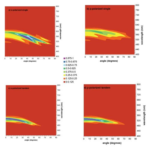
**Fig. 8** Emitted field intensity as a function of emission angle for the single microcavity OLED in (a) *s* and (b) *p*-polarizations. Emitted field intensity as a function of emission angle for the tandem microcavity OLED in (c) *s* and (d) *p*-polarization. The angle is measured in the *x*-*z* plane (Fig. 1) with respect to the surface normal. The *s*- and *p*-emission spectra are normalized by the same factor in the single and tandem plots.
