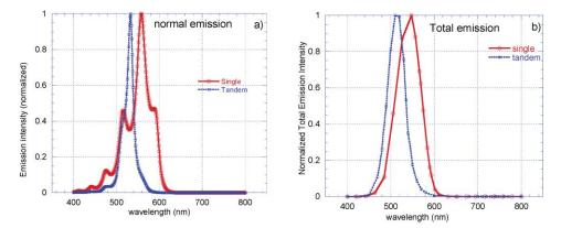
**Fig. 7** Simulated normal emission and total emission (over all angles) from microcavity tandem and single unit OLEDs. The source profile of  $Alq_3$  emission is utilized. Averaging is performed for dipole sources in the upper and lower unit cells.
