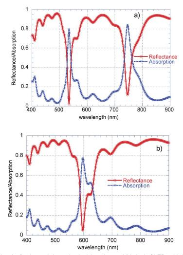
Fig. 6 Simulated reflection and absorption for (a) tandem and (b) single OLEDs with the scattering matrix method, showing the presence of microcavity modes.
