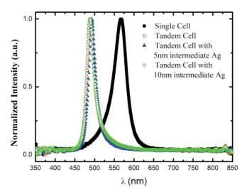
Fig. 2 The measured EL from microcavity single unit and tandem OLEDs with or without intermediate silver layers of varying thickness.
