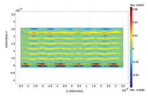
Fig. 5 Electric field intensity within the OLED, arising from the distribution of dipole sources within the organic emitting layer.
