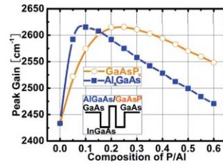
**Fig. 6** Influence of P/Al composition on peak gain in double-well structure.
