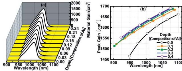
**Fig. 2** (a) Gain spectra and (b) peak gains as functions of emission wavelengths of the single-well structures with different depth.
