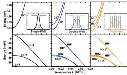
**Fig. 8** Band structures of single-, double-, and triple-well structures.
