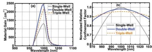
**Fig. 9** (a) Comparison of gain and (b) confinement factors of single-, double-, and triple-well structures.
