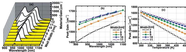
**Fig. 1** (a) Gain spectra, (b) peak gains as functions of emission wavelengths, and (c) peak gains versus temperature of the single-well structures with different width.
