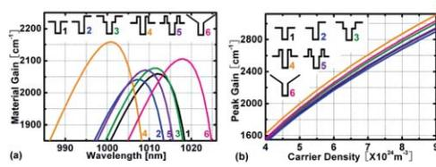
**Fig. 4** (a) Gain spectra and (b) peak gains versus carrier density of six different single-well structures.
