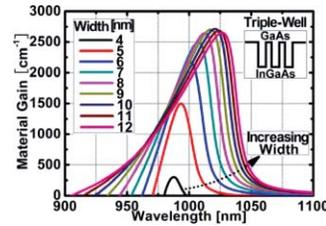
**Fig. 7** Gain spectra of different triple-well structures.
