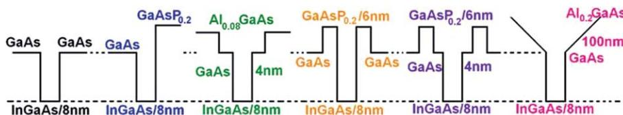
**Fig. 3** Configurations of six different single-well structures.
