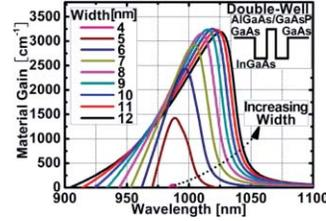
**Fig. 5** Gain spectra of double-well structures with different width.
