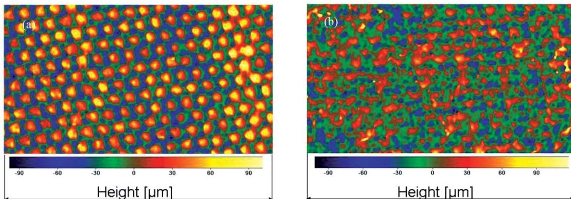
**Fig. 2** (a) Surface structure 3D-profilometry with the Primos system of polyamide fabric. (b) Surface structure 3D-profilometry with the Primos system of polyester fabric.
