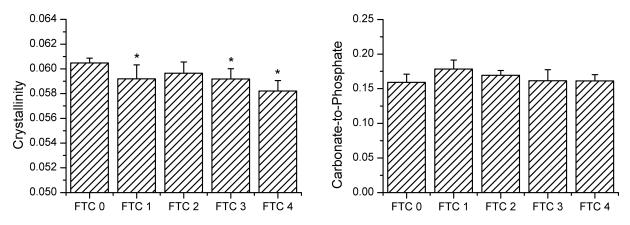
**Fig. 2** Crystallinity and carbonate-to-phosphate Raman measurements on cortical bone. Crystallinity showed decreased levels after one FTC and further decline after subsequent freezing and thawing while carbonate levels did not vary significantly. Asterisks are indicative of a Bonferonni pairwise difference from FTC 0 with significance of p < 0.05.
