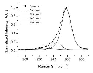
**Fig. 3** Nonlinear curve fitting results for the 882 to 982 cm<sup>-1</sup> region. Three Gaussian/Lorentzian functions were used to represent the phosphate 959 cm<sup>-1</sup> band and two matrix bands at 943 and 924 cm<sup>-1</sup>. Region was truncated to not include the phenylalanine band at 1002 cm<sup>-1</sup> and the proline and hydroxyproline bands at 853 and 876 cm<sup>-1</sup>. Fitting the band reveals the true symmetry of the underlying phosphate peak.
