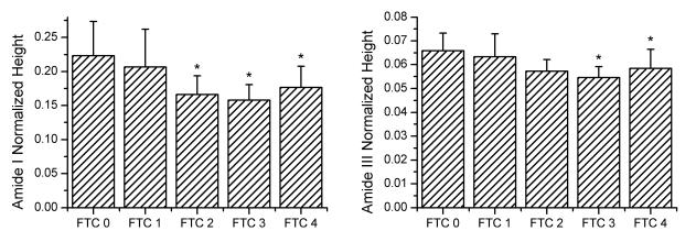
**Fig. 1** Raman measurements of the amide I and amide III band heights on cortical bone. Changes in band heights were first evident in amide I after FTC 2, and then in amide III after FTC 3. The FTC 1 group may also be indicative of subtle changes in the bone as it deteriorates. Asterisks are indicative of a Bonferonni pairwise difference from FTC 0 with significance of p < 0.05.
