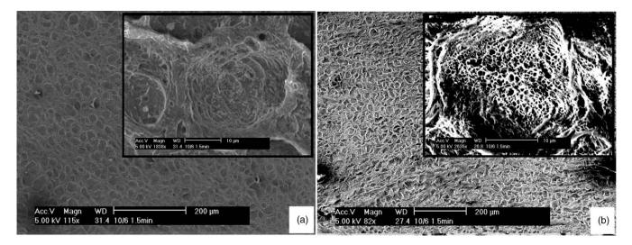
Fig. 5 Scanning electron microscopy of (a) outer surface of critical point during processed sample and (b) liquid nitrogen processed sample.
