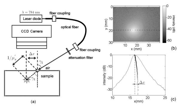
**Fig. 2** (a) Schematic of the oblique–incidence diffuse reflectance principle and setup. (b) Diffuse reflectance intensity map. (c) Diffuse reflectance profile (solid curve), calculated midpoint curve (dotted), and light entry point (dashed-dotted) at the position indicated in dashed line in (b).
