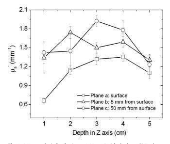
**Fig.** 7 Measured  $\mu'_s$  distribution at 784 nm inside the large PVA phantom. Data points represent average  $\mu'_s$  value of 5 measurements from the plane a, plane b and plane c of the phantom shown in Fig. 5. The error bars represent the standard deviations.
