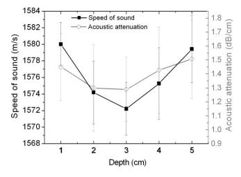
**Fig. 8** Speed of sound and acoustic attenuation (at 5 MHz) at different depths from the surface to the bulk of large PVA phantom at 22.5 °C. The data points represent the average values from 10 measurements, error bars represent the standard deviations.
