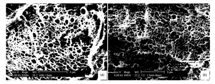
Fig. 9 Scanning electron microscope imaging of liquid nitrogen preprocessed specimens situated at (a) surface and (b) a deep lying cross-sections.
