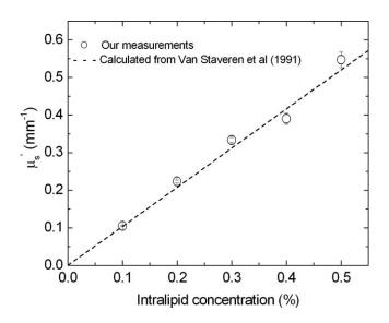
**Fig. 3** Reduced scattering coefficient ( $\mu'_s$ ) at 784 nm for varying Intralipid 20% concentrations in water measured using the obliqueincidence diffuse reflectance setup. Our results are compared with  $\mu'_s$  values calculated from Van Staveren et al.<sup>23</sup> Each sample is measured 5 times, error bars represent standard deviations.
