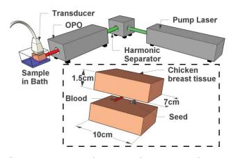
**Fig. 1** System setup. Surelite III pump laser pumps Surelite OPO Plus optical parametric oscillator (Continuum, Santa Clara, California) providing tunable light at 650 to 900 nm. Incident light interrogates the sample which is in a water bath beneath the 128-element L7-4 38 mm (5 MHz center frequency, ~70% fractional bandwidth) linear array transducer (AT5L40B, Broadsound Corporation, Jupei City, Hsinchu, Taiwan). Inset: blown up sample setup with relevant dimensions.
