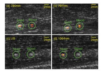
Fig. 2 (a) and (b) Combined ultrasound-photoacoustic images at a laser fluence of 20 mJ/cm<sup>2</sup> and a laser penetration depth of 2 cm. (c) and (d) Ultrasound and combined ultrasound-photoacoustic images at a fluence of 100 mJ/cm<sup>2</sup> and a laser penetration depth of 5 cm.
