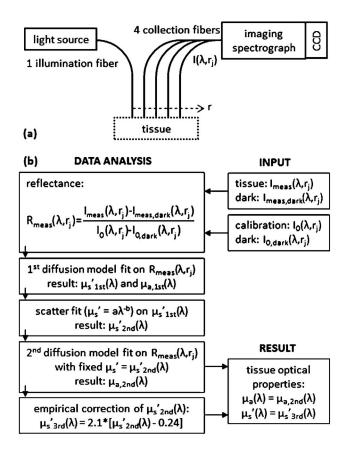
**Fig. 1** (a) Illustration of the measurement setup. (b) Schematic illustration of the data analysis.
