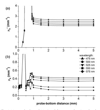
**Fig. 3** Measured values of (a)  $\mu'_{s}$  and (b)  $\mu_{a}$  as a function of probebottom distance for the 1.5% Intralipid-0.5% dye phantom and the black bottom layer. Results are shown for the wavelengths 475, 500, 525, 550, and 575 nm.
