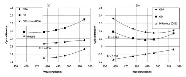
**Fig.** 7 Plots comparing  $OD_A$ ,  $OD_5$ , and OD for (a) the swine eye and (b) human eye.  $OD_A$  is calculated using [Hb] = 15 g/dL, extinction coefficients from Zijlstra et al. (Ref. 39), and the respective SO<sub>2</sub> values reported in this paper.
