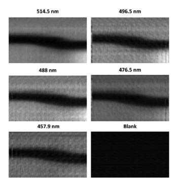
Fig. 4 Deinterlaced images of swine retinal vessel at five wavelengths and a blank.
