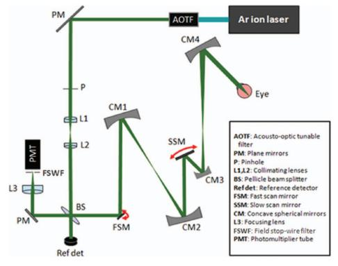
Fig. 2 Schematic of the ROx-3.
