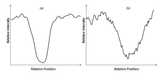
Fig. 5 Intensity profiles of (a) swine vessel and (b) human vein cross sections demonstrating the absence of significant glints.
