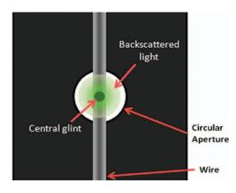
Fig. 3 Field stop-wire filter designed to reject the central vessel glint and transmit the backscattered light that contains hemoglobin information.
