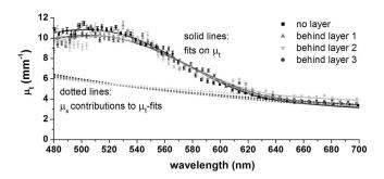
**Fig. 1** Measured  $\mu_t$  (dots) of a 1% Intralipid-10% dye phantom behind no layer and three TiO<sub>2</sub>-silicon layers (1:  $D = 155 \ \mu m$ ,  $\mu_t = 2.5 \ mm^{-1}$ ; 2:  $D = 170 \ \mu m$ ,  $\mu_t = 5 \ mm^{-1}$ ; 3:  $D = 355 \ \mu m$ ,  $\mu_t = 2.5 \ mm^{-1}$ ). Fits on  $\mu_t$ , and  $\mu_s$ -contributions to the  $\mu_t$ -fits are shown for all measurements.
