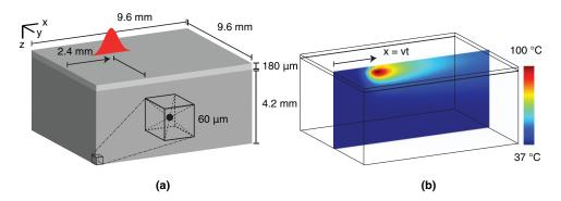
**Fig. 2** Finite difference simulation of the heat transfer equation. (a) Dimensions and layout of the simulation. A control volume approach with centered node-points was used. Instead of scanning the beam, after each time iteration the tissue volume was moved along the x-coordinate. (b) Resulting spatiotemporal heat profile.
