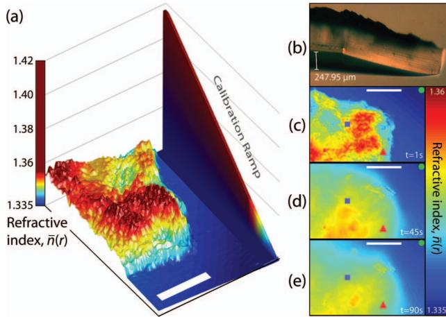
**Fig. 1** Two-dimensional absolute refractive index maps of a CSIC film during dissolution at (a, c)  $t = 1$  s, (d)  $t = 45$  s, and (e)  $t = 90$  s. Scale bar represents  $200 \mu\text{m}$ . (b) Representative image of the PDMS calibration ramp. Plots in Fig. 2 come from the purple squares, red triangles, and green circles seen in (c–e). (a) is a still image from Video 1 (QuickTime, 6.2 MB). [URL: <http://dx.doi.org/10.1117/1.3665439.1>]
