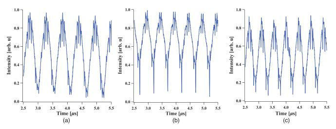
**Fig. 2** Experimental time traces of the QCL output when external OF is applied to the QCL and with a sine modulation of the continuous bias of: (a) 1.8 MHz, (b) 2 MHz, and (c) 2.2 MHz; all of the traces were retrieved for a continuous bias of 430 mA and a modulation amplitude of 120 mA, but only the one in the middle exhibits dropouts with a magnified amplitude, which is, however, not enough to categorize them as extreme events.
