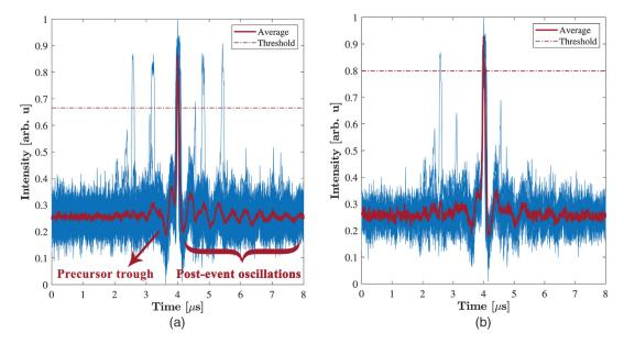
**Fig. 5** (a) Time series centered on the maximum of local bursts and superposition of 37 extreme events. The corresponding averaged output power is displayed with a purple solid line and the threshold corresponding to an abnormality of 2 is displayed with a dash-dot line. (b) Same data plot but for 13 extreme events surging above an abnormality index of 2.4. In the left panel, the trough preceding the optical burst, as well as the oscillations following the extreme event, is underlined.
