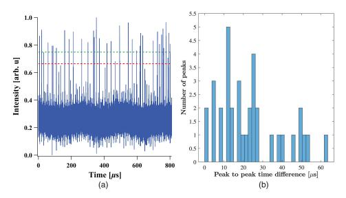
**Fig. 3** (a) Experimental time trace with extreme events and associated thresholds for the two criteria. The dashed red line represents the threshold corresponding to criterion  $C_1$  (H=0.665) and the dashed green line represents the threshold corresponding to criterion  $C_2$  (H=0.749). Events with their maximum above these dashed lines are considered as extreme. (b) Histogram of the time intervals between extreme events in the case where the  $C_1$  criterion is applied to the time trace.
