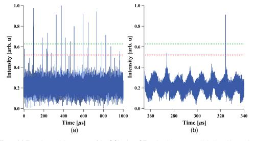
**Fig. 6** (a) Experimental time traces of the QCL when OF and a sine wave modulation with a period of 10  $\mu$ s and an amplitude of 4 mA are applied. The dashed red line represents the  $C_1$  criterion and the dashed green line represents the  $C_2$  criterion. (b) Close-up on extreme events and the low-amplitude sine modulation, revealing that extreme events can only occur on top of the periodic modulation.
