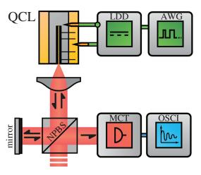
**Fig. 1** Experimental setup with an external cavity for the OF via a mirror. NPBS, nonpolarizing beam splitter; MCT, mercury–cadmium–telluride detector; OSCI, fast oscilloscope; AWG, arbitrary waveform generator; LDD, laser diode driver.
