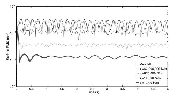
Fig. 6 The effects of mechanism stiffness on the impulse response.
