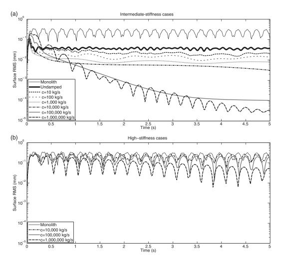
Fig. 8 The effects of damping on the impulse response for (a) intermediate- and (b) high-stiffness mechanisms.
