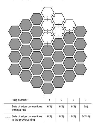
**Fig. 3** Mechanism totals by ring number. The total number of mechanisms depends on the number of mechanisms used to connect a pair of adjacent edges,  $n_e$ , as well as the number of edge pairs. For ease of counting, the edge pairs are divided into two categories: in-ring pairs, for segments in the same ring, and cross-ring pairs, for segments in rings *i* and *i* – 1. For a mirror with  $n_r$  rings, there are  $9n_r^2 + 3n_r$  pairs, for a total of  $n_e(9n_r^2 + 3n_r)$  mechanisms.
