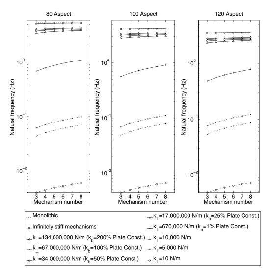
Fig. 4 The first natural frequency as a function of aspect ratio, mechanism number, and mechanism stiffness.
