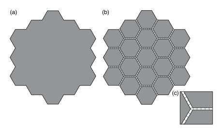
**Fig. 2** Mirror modeling. In the finite-element model, a mirror is composed of rings of hexagonal segments, with the connectivity determining whether the mirror is monolithic or segmented. For a monolithic mirror (a), the segments are connected continuously along the edges, while for an edgewise-connected mirror (b), the segments are connected at discrete locations by collections of damped springs that represent the mechanisms (c).
