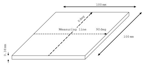
Fig. 3 Schematic view of the flat substrate sample and measuring line.
