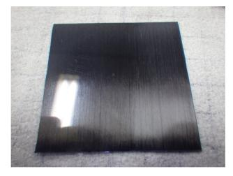
Fig. 2 Photograph of the carbon fiber reinforced plastic (CFRP) flat substrate.
