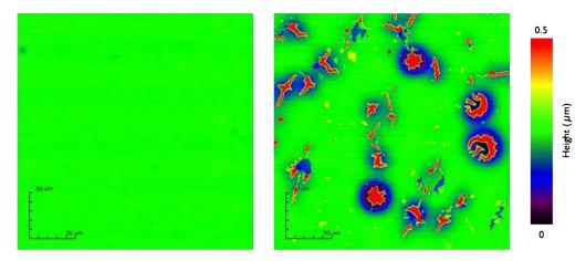
Fig. 8 The images of the SiOx COP sample surface observed by OLS4000 with a  $50\times$  objective lens. The left image was acquired at the start of the moisture absorption test at  $60^{\circ}$ C with RH of 100%, while the right image was acquired at a duration time of 900 h.
