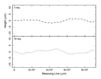
Fig. 4 Surface waviness of the flat substrate sample. The dashed line is the surface waviness with a cutoff wavelength of 8000  $\mu$ m at the center-line that is parallel to 0 deg, and the dotted line is the waviness of center-line parallel to 90 deg.
