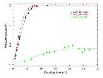
**Fig. 5** Time profiles of the moisture content of the CFRP substrate in the accelerated moisture absorption aging test. Black points represent the environment at 60°C with relative humidity (RH) of 100%, red points represent 80°C with RH of 100%, and green points represent the laboratory environment. The dashed lines are the fitting results using Fick's law [Eq. (2)].
