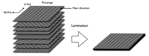
**Fig. 1** A schematic view of the quasi-isotropic lamination and the definition of the fiber direction angle. This shows 8-ply lamination of [0/45/-45/90]s.
