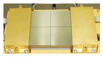
Fig. 6 Photograph of the flight CCDs mounted on the cold plate.
