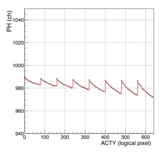
**Fig. 15** PH of the Mn-K $\alpha$  line at 5.9 keV as a function of ACTY. The function shown with the red curve is the same one as used by Nobukawa et al. <sup>36</sup> The plotted data are from CCD3 Segment AB, where no CTI anomaly is found.
