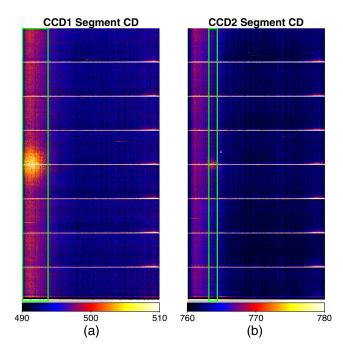
**Fig. 17** Dark frames from (a) CCD1 segment CD and (b) CCD2 Segment CD taken at −120°C. The green rectangles denote the regions used for the plots shown in Fig. 16. The rows in white are those with charge injection.
