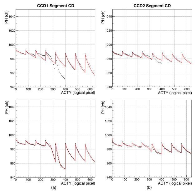
**Fig. 16** Same as Fig. 15 but from (a) CCD1 segment CD and (b) CCD2 segment CD. The analyzed regions are shown in Fig. 17. The data are fit with the function proposed by Nobukawa et al.<sup>36</sup> and the modified function (see text) in the top panels and bottom panels, respectively.
