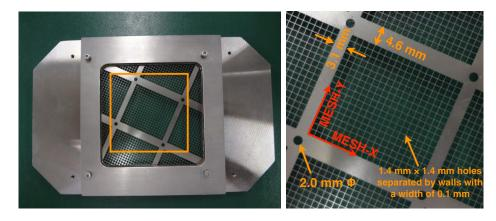
**Fig. 12** Photograph of the stainless steel mesh in a look-down view. The right photograph is a zoom-in view of the region enclosed by the orange square in the left photograph. The definition of the MESH coordinate is indicated in red.
