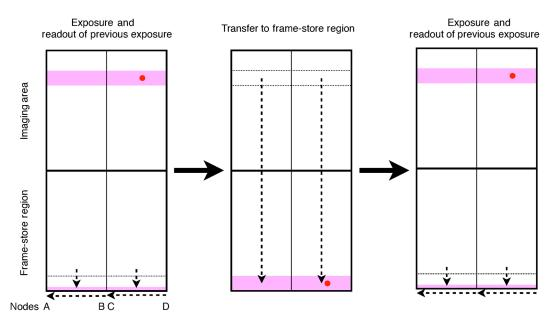
Fig. 8 Schematic diagram of the window option operation.
