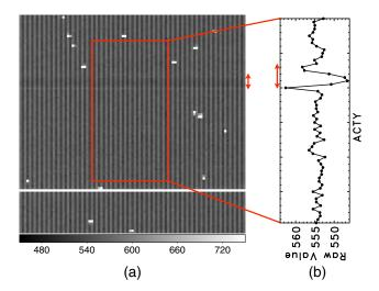
**Fig. 10** (a) Raw frame data from a  $\sim$ 100  $\times$  100 logical pixel region of CCD3 segment AB taken in an on-ground test and (b) projection of the frame along the ACTY direction. The white row in the frame image is a charge injection row. Pixel values of the rows indicated with the red arrows become significantly higher/lower than those of the other rows. This phenomenon was found to be synchronized with a rapid change of the heater current.
