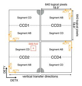
**Fig. 7** Schematic layout of the CCD arrays in a look-up view. Only the imaging areas are drawn. The red cross and square indicate the aim point of SXT-I and the FoV of the SXS, respectively. The gray-shaded zones are approximate locations illuminated by the <sup>55</sup>Fe calibration sources. The definitions of the DET and ACT coordinates are indicated in black and orange, respectively.
