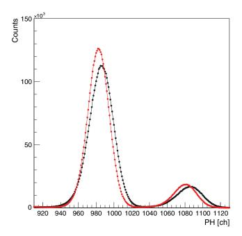
**Fig. 19** Spectra of Mn-Kα and Kβ x-rays from <sup>55</sup>Fe taken with CCD1 Segment CD before (black) and after (red) the trail and CTI corrections. Events with grades 0, 2, 3, 4, and 6 are selected. Here the peaks are shifted toward lower energies after the corrections since PH<sub>5.9 keV</sub> is set to 982 ch.
