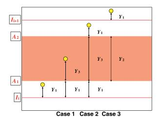
**Fig. 18** Definitions of  $Y_1$ ,  $Y_2$ , and  $Y_3$  in the case where a CTI anomaly (the shaded region) from ACTY =  $A_1$  to ACTY =  $A_2$  is between the two charge injection rows (the red horizontal lines) at ACTY =  $I_i$  and ACTY =  $I_{i+1}$ .
