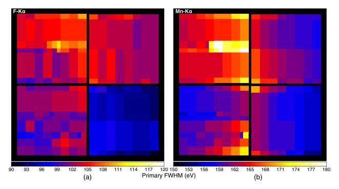
**Fig. 22** Maps of widths in FWHM of the primary peak (a) at 0.68 keV and (b) at 5.9 keV in the DET coordinate. This result is reflected in the detector response function used for observational data analysis.
