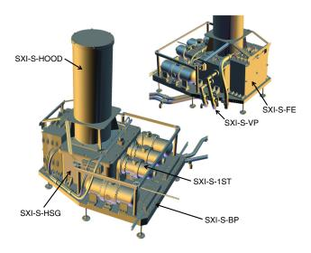
Fig. 2 External views of SXI-S from different angles.
