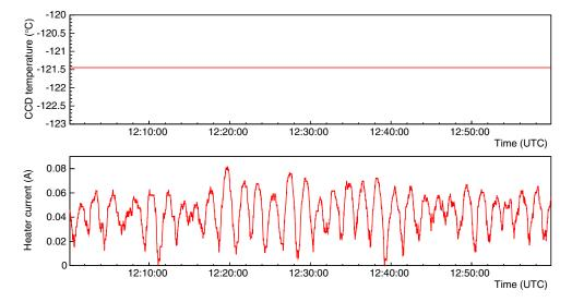
Fig. 11 Time history of the CCD temperature and the heater current obtained in an on-ground test. The targeted temperature was set to  $-121.4^{\circ}$ C. The measured temperature was actually stabilized at the targeted temperature within one digit of the data, which corresponds to  $\sim 0.1^{\circ}$ C.
