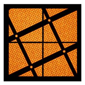
**Fig. 13** X-ray shadow image of the mesh by the SXI CCD array in the DET coordinate defined in Fig. 7 (in a look-up view). We irradiated the CCDs with Mn-K $\alpha$  at 5.9 keV and K $\beta$  at 6.5 keV from an  $^{55}$ Fe source. The image is smoothed with a Gaussian kernel with  $\sigma=$  1.5 logical pixels.
