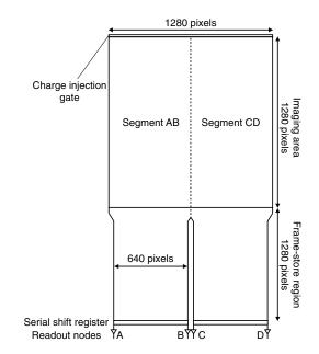
Fig. 4 Schematic view of the CCD, Pch-NeXT4. The segments AB (CD) are read out either from the readout node A or B (C or D).
