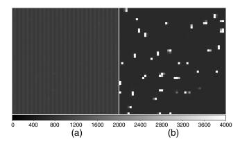
**Fig. 23** Dark frames taken in (a) May 2013 and (b) September 2014 with optical light illumination. Shown are the same  $\sim 50 \times 50$  logical pixel region of CCD4 Segment AB. The white pixels in the right panel are those with pinholes in the OBL. The pixel values reflect the optical light transmission in linear scale.
