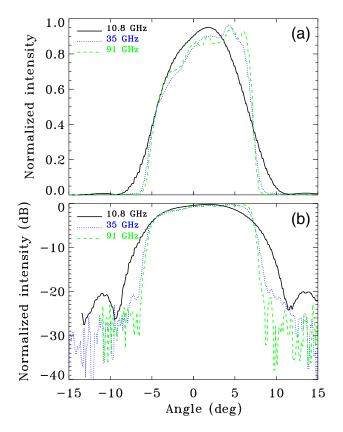
**Fig. 5** Comparison of copolar beam patterns as a function of frequency for the  $\hat{u}$  polarization along the +45 deg slice. Beam patterns are shown for both (a) a linear scale and (b) logarithmic scale. Diffraction broadens the beam pattern at the lowest frequency, but the beam shape is nearly constant at higher frequencies.
