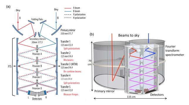
**Fig. 1** (a) Schematic view of the PIXIE optical signal path. A polarizing FTS interferes the signal from two copointed beams to produce a fringe pattern proportional to the difference spectrum between orthogonal polarization states from the two beams. Polarization-sensitive detectors mounted within multimoded concentrators sense the fringe pattern. (b) Physical layout of PIXIE optics.
