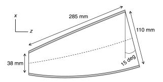
**Fig. 2** Schematic of the rectangular concentrator in the  $\hat{x} - \hat{z}$  plane. The dashed line indicates the junction of the  $\hat{u}$  and  $\hat{v}$  walls, which project out of the plane of the page (see text). Dimensions are for the larger scaled concentrator used to measure the beam patterns; the concentrator for the actual instrument is three times smaller in all dimensions.
