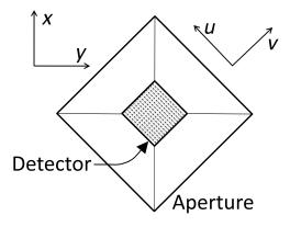
**Fig. 3** Schematic view looking into the concentrator aperture from the FTS, showing the instrument (*xy*) and concentrator (*uv*) coordinate systems. The concentrator is rotated 45 deg with respect to instrument coordinates so that asymmetries in instrument coordinates affect both detectors equally. Dashed lines show the orientation of the absorbing grid for the  $\hat{u}$  detector.
