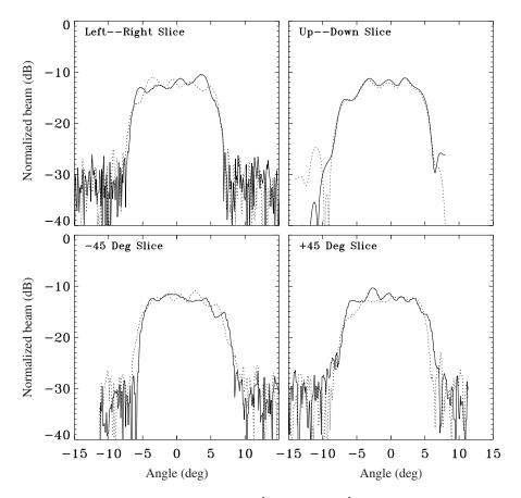
**Fig. 6** Comparison of crosspolar beam patterns for  $\hat{u}$  (solid line) and  $\hat{v}$  (dotted) polarization measured at 35 GHz for the scaled concentrator. Beam slices are the same as Fig. 4.
