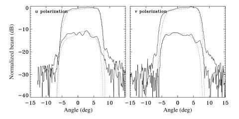
**Fig. 7** Comparison of measured beam patterns at 35 GHz (solid lines) to the model including effects of diffraction and the number of modes (dotted lines). The upper set of curves show the copolar beam while the lower set shows the crosspolar response. The primary effect of the crosspolar response is a 5% loss in polarization efficiency.
