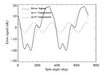
**Fig. 8** Systematic error for the 35-GHz crosspolar response convolved with simulated CMB maps. The crosspolar response (solid line) is dominated by an m = 1 dipole component (dotted line), which does not contribute to the reconstructed sky polarization. The m = 2 component (dashed line) creates a systematic error in polarization, but is small compared to the r = 0.01 inflationary signal.
