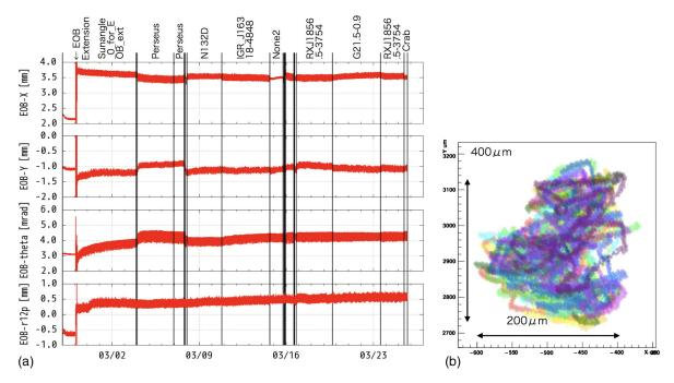
**Fig. 3** (a) The time history of the center position of the EOB (EOB-X and EOB-Y), its rotation around the spacecraft Z-axis (the launch direction) from the nominal orientation, and changes of the distance between the two corner cubes. (b) Stability of the focal plane alignment measured in about a day with CAMS after the EOB extension.
