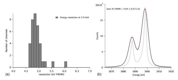
**Fig. 6** (a) A histogram of the distribution of resolutions measured across the array. (b) The whole-array spectrum around 5.9 keV. The points are the data, with sqrt(N) error bars on the counts barely visible. The dark line is the best fit to a model of the natural line shape convolved with Gaussian broadening, and the dashed gray line is the natural line shape.
