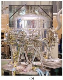
**Fig. 5** Photographs of (a) SXS sensor and (b) SXS dewar. The sensor was suspended from the outer structure using Kevlar, and electrical connections to the housing were made using tensioned wires to reduce the sensitivity to microphonics. The outer shell of the dewar is 950 mm in diameter.
