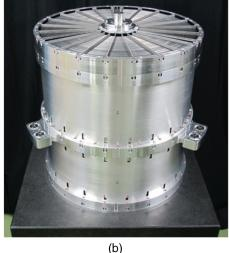
**Fig. 4** Photographs of flight models of (a) Soft X-ray Telescope, SXT-S, and (b) Hard X-ray Telescope, HXT-1.
