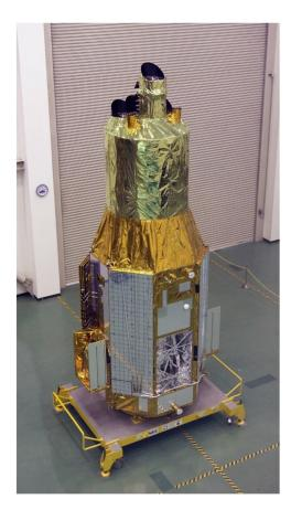
**Fig. 1** A photograph of the Hitomi satellite. The height in this launch configuration is 7.86 m.
