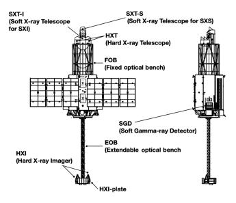
**Fig. 2** Schematic view of the Hitomi satellite with the extensible optical bench deployed. The total length of the satellite is about 14 m.<sup>8,10–12</sup> The SXS instrument is equipped in the opposite side of the solar paddle.
