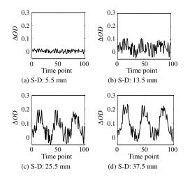
Fig. 7  $\Delta$ OD measured at each S-D distance as upper and lower layers driven in white-noise and CBV waveform, respectively (condition 1). S-D distances: (a) 5.5 mm, (b) 13.5 mm, (c) 25.5 mm, and (d) 37.5 mm.
