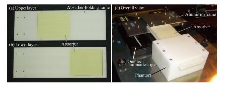
Fig. 1 Photos of the developed phantom. (a) Upper layer and (b) lower layer of absorber-holding frame. (c) Overall view of dynamic phantom.
