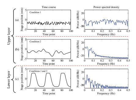
Fig. 6 Time course and power spectrum density (PSD) of stage-position change simulating NIRS signal when one point of time course data was equivalent to 1 sec: (a) white noise, (b) biological fluctuation, and (c) cerebral blood volume (CBV) response evoked by neuronal activation.
