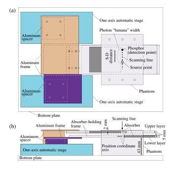
**Fig. 2** Structure of phantom and driving mechanism of absorbers. (a) Top view. (b) Front view. Each absorber-holding frame is independently controlled by a corresponding one-axis automatic stage.
