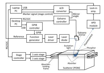
**Fig. 3** Block diagram of multidistance NIRS system and stage controller for phantom. Two one-axis stages are independently driven by a stage controller that is commanded by a laptop PC through RS232C.
