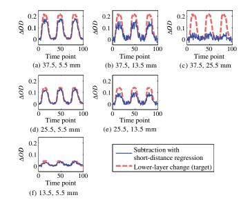
**Fig. 8** Subtraction result with short-distance regression of  $\Delta$ OD measured while both layers are driven in condition 1, and  $\Delta$ OD measured at a long distance while only lower layer (target) is driven. Combination of S-D distances: (a) 37.5 and 5.5 mm, (b) 37.5 and 13.5 mm, (c) 37.5 and 25.5 mm, (d) 25.5 and 5.5 mm, (e) 25.5 and 13.5 mm, and (f) 13.5 and 5.5 mm.
