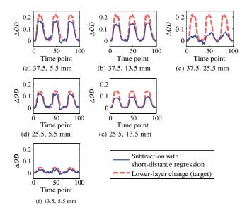
**Fig. 10** Subtraction result with short-distance regression of  $\Delta$ OD measured while both layers were driven in condition 2, and  $\Delta$ OD measured at a long distance while only lower layer (target) was driven. Combination of S-D distances: (a) 37.5 and 5.5 mm, (b) 37.5 and 13.5 mm, (c) 37.5 and 25.5 mm, (d) 25.5 and 5.5 mm, (e) 25.5 and 13.5 mm, and (f) 13.5 and 5.5 mm.
