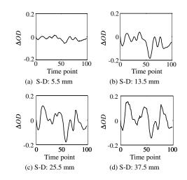
Fig. 9  $\Delta$ OD measured at each S-D distance as upper and lower layers were driven in waveform of biological fluctuation and CBV, respectively (condition 2). S-D distances: (a) 5.5 mm, (b) 13.5 mm, (c) 25.5 mm, and (d) 37.5 mm.
