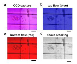
**Fig. 3** Simultaneous imaging of murine fibroblast cells flowing through two perpendicular microchannels separated by  $300 \,\mu$ m. (a) Composite color CCD image acquired in a single exposure. (b,c) Color separation of the image in (a) provides information of the cells flowing in each individual microchannel. (d) Focus stacking of the images from (a) into a single image where out of focus information can now be removed. Scale bars,  $100 \,\mu$ m.
