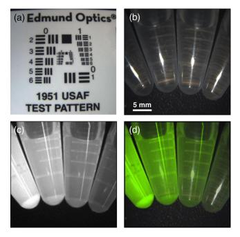
**Fig. 5** Bench testing for the imaging system. (a) Color image of USAF 1951 resolution test target acquired at 5 cm working distance. (b–d) Color, NIR, and merge images of indocyanine green (ICG) in dimethyl sulfoxide (DMSO), respectively, at 1.0  $\mu$ M, 0.5  $\mu$ M, 0.25  $\mu$ M, and 0.125  $\mu$ M (left to right). Note the accurate registration of images from the color and NIR channels.
