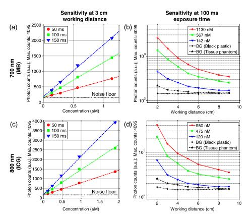
**Fig. 7** Sensitivity performance evaluation. (a) Average fluorescence signal from various concentrations of methylene blue (MB) in DMSO at 3 cm working distance. (b) Photon counts measured from MB in DMSO at three concentrations at varying working distances. (c) Average fluorescence signal from various concentrations of ICG in DMSO at 3 cm working distance. (d) Photon counts measured from ICG in DMSO at three concentrations at varying working distances. BG, background.
