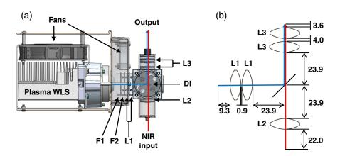
**Fig. 2** Source coupler design. (a) Mechanical layout of the source coupler mounted on the custom white light source chassis. F1: IR filter. F2: 650SP filter. L1: 30 mm biconvex lens. L2: 25 mm biconvex lens. Di: T673LP dichroic mirror. L3: 25 mm biconvex lens. (b) Optical design of source coupler.
