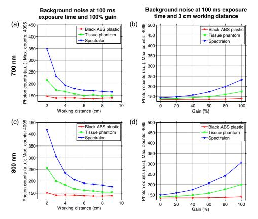
**Fig. 6** Background noise evaluation using three different reflectance materials (black ABS plastic, tissue phantom, and Spectralon). (a and b) Background noise measured in the 700-nm channel under 660-nm excitation and white light at their maximum output, as a function of working distance and gain. (c and d) Background noise measured in the 800-nm channel under 760-nm excitation and white light at their maximum output, as a function of working distance and gain.
