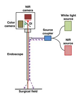
Fig. 1 Schematic of a typical dual-channel near-infrared (NIR) and color endoscopic imaging system. Light from a filtered white light source is combined with the light from an NIR excitation source and injected into the endoscope through the illumination port. Light is collected through the endoscope imaging channel, split using a dichroic mirror (Di) and filtered in two channels, one for the color imaging and the other for the NIR fluorescence imaging.
