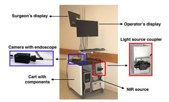
**Fig. 4** The NIR-optimized dual-channel clinical endoscopic imaging system. The system comprises of a white light and NIR laser source, a dual-channel camera, a rigid endoscope, and a computer for data acquisition and system control housed in a small form-factor cart for easy transportation. Note the two displays, one for the system operator and the other for the surgeon.
