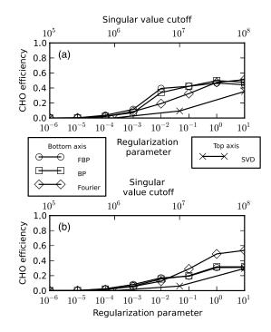
**Fig. 8** CHO efficiency for the (a) constant *Q* channels and (b) DOG channels for the 0.5-mm cube SKE/BKE task.
