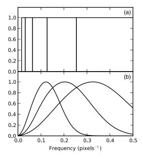
Fig. 6 Channel profiles for (a) constant Q channels and (b) DOG channels.
