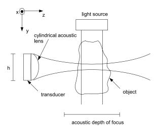
Fig. 1 Geometry of photoacoustic imaging system.
