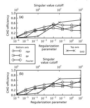
**Fig. 9** CHO efficiency for the (a) constant *Q* channels and (b) DOG channels for the point source SKE in a lumpy background task.
