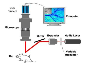
Fig. 1 Schematic of the laser speckle contrast imaging system.
