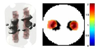
**Fig. 9** Fluorescence yield *f* reconstructed from simulated data using Tikhonov regularization and  $S_{1024}$  in (left) 3-D and (right) 2-D cross section at z = 0 mm.
