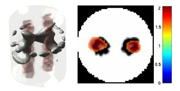
**Fig. 8** Fluorescence yield *f* reconstructed from simulated data using Tikhonov regularization and data compression in (left) 3-D and (right) 2-D cross section at z = 0 mm.
