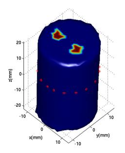
**Fig. 3** Geometry used in the simulations. The FEM mesh is generated from X-ray CT images of the experimental phantom. The asterisk markers indicate the source positions.
