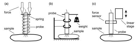
Fig. 2 Diffuse reflectance systems for *in vivo* measurements based on a calibrated spring (a), calibrated weights (b), or a motorized linear stage (c).
