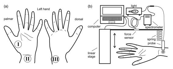
**Fig. 3** (a) Three selected measurement sites: (I) above abductor pollicis brevis muscle, (II) in the middle of the wrist crease above the veins, and (III) at the lateral part of the wrist above ulnar styloid process. (b) Experimental measurement system.
