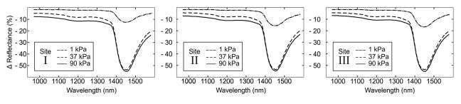
Fig. 4 Relative reflectance change as a function of the contact pressure (1, 37, and 90 kPa) for the three selected measurement sites.
