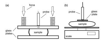
Fig. 1 Diffuse reflectance systems for *ex vivo* measurements based on calibrated springs (a) or a scale (b).
