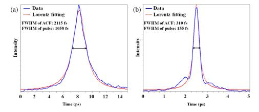
Fig. 2 Auto correlation function (blue, solid line) and its Lorentz fitting (red, dot line) are shown: (a) without a prism pair and (b) after negative chirping with a prism pair.
