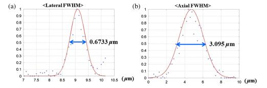
Fig. 6 Resolution test results with fluorescent beads of 170-nm diameter: (a) the measurement result of lateral full-width at half-maximum (FWHM) and (b) the measurement result of axial FWHM.
