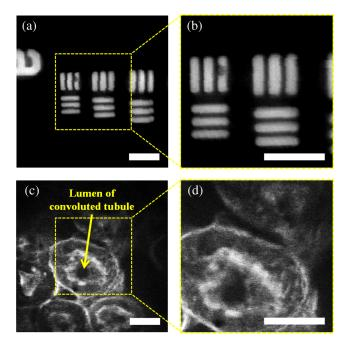
**Fig. 7** (a) The image of 1951 USAF test target (group 7, element 4, 5, and 6); (b) two times magnified image of (a) obtained by partial scanning; (c) the image of mouse kidney section; and (d) two times magnified image of (c) obtained by partial scanning. The lumen of the convoluted tubule is marked with yellow arrows. Scale bar is 20  $\mu$ m.
