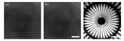
**Fig. 5** Reflection images of test targets (R1L3S5P, Thorlabs): (a) image of a distortion grid with the period of 5  $\mu$ m; (b) reconstructed image of (a); and (c) reconstructed image of a Siemens star target with 100- $\mu$ m diameter center circle. Scale bar is 20  $\mu$ m.
