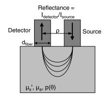
Fig. 1 Schematic of the two-fiber reflectance geometry.
