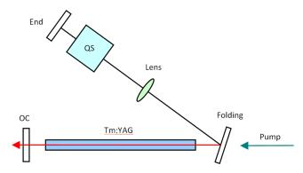
Fig. 2 Custom-made Q-switched (QS) Tm:YAG laser. Conventions: End—end mirror, QS—Q-switch, Lens—lens, Folding—folding mirror, Pump—pump beam, and OC—output coupling mirror.
