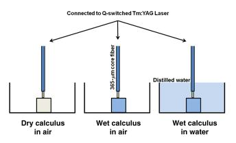
Fig. 4 Three experimental conditions: dry calculus in air, wet calculus in air, and wet calculus in water.
