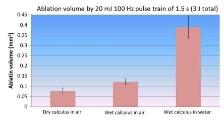
Fig. 6 Calculus ablation volume under three different conditions.
