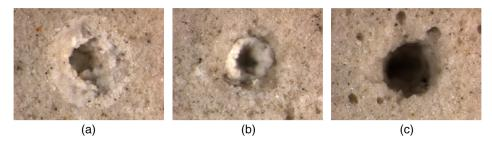
Fig. 5 Typical screenshots of laser ablation areas under different sample conditions by Leica M205C series stereomicroscope: (a) dry sample; (b) wet sample; and (c) in-water sample.
