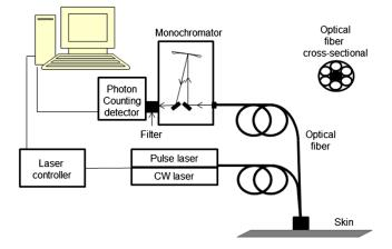
Fig. 1 Experimental setup for skin autofluorescence lifetime measurements.
