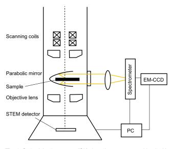
**Fig. 1** Cathodoluminescence (CL) detection system combined with a scanning transmission electron microscopy (STEM) instrument.
