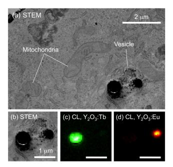
**Fig. 5** STEM and CL images of  $Y_2O_3$ : Eu and  $Y_2O_3$ : Tb nanophosphors in 100 nm thin section of HeLa cell. (a) STEM image of 100 nm thin section of HeLa cell with introduced nanophosphors, (b) partial view of STEM image of HeLa cell with introduced nanophosphors, (c) and (d) CL images of nanophosphors ( $Y_2O_3$ : Eu and  $Y_2O_3$ : Tb) in a cell.
