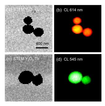
**Fig. 4** STEM and CL images of  $Y_2O_3$ : Eu and  $Y_2O_3$ : Tb nanophosphors synthesized by HP method. (a) and (b) Interlaced STEM image and CL image of  $Y_2O_3$ : Eu. (c) and (d) Interlaced STEM image and CL image of  $Y_2O_3$ : Tb.
