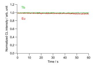
Fig. 3 Stability of CL intensity against electron beam exposure  $(Y_2O_3:Eu$  nanophosphors synthesized by homogeneous method).
