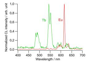
**Fig. 2** Spectra of  $Y_2O_3$ : Tb and  $Y_2O_3$ : Eu nanophosphors synthesized by homogeneous precipitation (HP) method (slit size: 0.1 nm, blaze wavelength: 400 nm, groove density: 150 L/mm).
