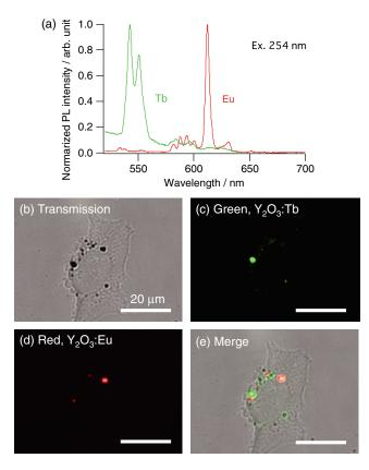
**Fig. 6** (a) Emission spectra of  $Y_2O_3$ : Eu,  $Y_2O_3$ : Tb, (b) transmission, (c) green fluorescence, (d) red fluorescence, and (e) merged images of  $Y_2O_3$ : Eu and  $Y_2O_3$ : Tb nanophosphors contained in a HeLa cells.  $Y_2O_3$ : Eu, and  $Y_2O_3$ : Tb nanophosphors were excited by 254-nm UV light
