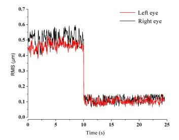
**Fig. 4** The representative time course of total root mean square (RMS) aberration for both eyes. The black and red lines represent RMS aberration for the right eye and the left eye, respectively. AO is initiated at T = 10 s.
