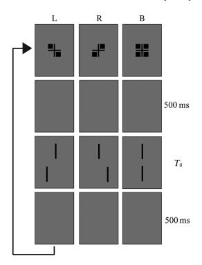
Fig. 3 The time sequence of a typical trial in stereoacuity tests. The columns "L" and "R" are visual displays for the left eye and the right eye, respectively. With accurate binocular fusion, the subject would perceive just as "B" shows.
