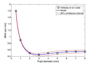
**Fig. 1** Best corrected (zero blur) MAR as a function of pupil diameter as given by Holladay et al. (circles), and fit of these data to the model function  $MAR_H(D)$  plotted as a continuous line (blue in color). The 95% confidence interval of the model is also plotted as two dashed lines (red in color).
