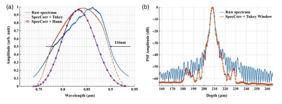
Fig. 4 (a) Spectral shape correction and apodization effects on the source spectrum. (b) The suppression of sidelobes and noise floor of the axial PSF after applying Tukey window for apodization.
