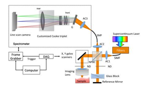
**Fig. 1** Schematic of SD-OCT system. SMF, single mode fiber; AC, achromatic lenses; ND, neutral density filter; NPBC, nonpolarized beam cube; G, transmission diffraction grating. All optical components were chosen to have antireflection coating for 600 to 1000 nm to minimize loss. Inset: schematic of the spectrometer with customized focusing optics.
