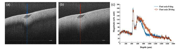
Fig. 11 Penetration depth and signal attenuation with respect to incident polarization state alignment. (a) Fast-axis of half-wave plate was set to 0 deg. (b) Fast-axis of half-wave plate was set to 20 deg. (c) 20-pixel averaged A-line profiles taken at the regions marked with arrows in (a) and (b). Scale bar: 100  $\mu$ m.
