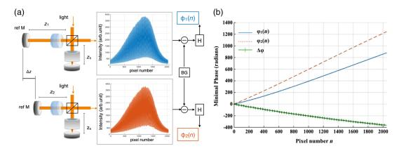
**Fig. 3** (a) Spectrometer calibration process. Interferograms for two different optical path differences were generated with background subtraction. Phase information was extracted from the analytical signal constructed by Hilbert transform. (b) The minimal phases constructed from the interferogram with respect to the pixel number. The phase difference (green) of the two interference signals was fitted to a third-order polynomial as a pixel calibration metric for linear-*k* redistribution.
