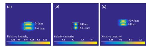
**Fig. 2** PSFs for two wavelengths with a spectral separation of 0.1 nm at (a) 740, (b) 840, and (c) 940 nm. The FWHM of the PSF was 7.4, 9.4, and 10.6  $\mu$ m for 740, 840, and 940 nm, respectively. The color bar shows the relative intensity. The yellow boxes indicate the location and physical dimensions of two adjacent rectangular pixels (14  $\mu$ m × 28  $\mu$ m).
