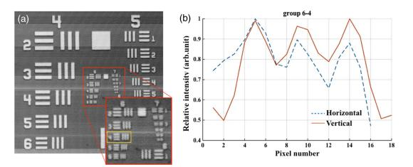
**Fig. 6** Lateral resolution calibration with a USAF1951 target. (a) An averaged *en face* image generated from a 3-D OCT volume by extracting the orthogonal slices with respect to the depth direction. The inset shows a zoom-in view of groups 6 and 7. The last group with distinguishable line group (group 6-4) is highlighted in the yellow box. (b) The averaged pixel profiles extracted across the horizontal (blue dashed line) and vertical (red solid line) bars of group 6-4.
