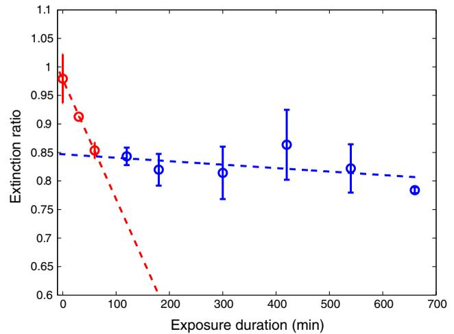
**Fig. 3** Variation of the extinction ratio as a function of duration of tooth exposure to acid (in minutes). Error bars correspond to the standard deviation. Circles correspond to experimental data. Lines are guides for the eyes.
