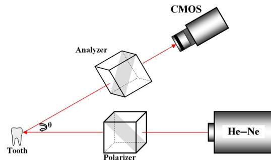
**Fig. 2** Overview of the speckle experimental setup.
