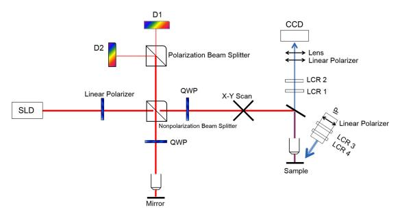
Fig. 1 Combined PS-OCT and Mueller matrix polarimeter schematic.
