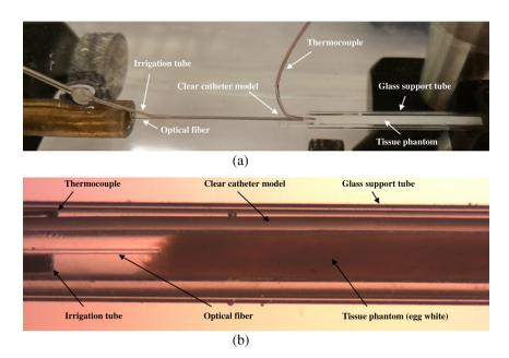
**Fig. 2** (a) Photograph of tissue ablation setup in submerged saline bath. (b) Magnified image of catheter model with 100- $\mu$ m core (170- $\mu$ m OD) TFL fiber and 320- $\mu$ m ID (370- $\mu$ m OD) irrigation tube.
