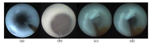
**Fig. 8** Images from 0.7-mm OD, 10,000 pixel endoscope, simulating an image-guided laser ablation procedure. (a) Clear catheter near distal tip with CSF drainage holes and side-by-side 100- $\mu$ m core fiber. (b) Clear catheter at distal tip with radiopaque plug. Egg white sample prepared in opaque white commercial catheter with side-by-side 100- $\mu$ m core fiber and 370- $\mu$ m OD irrigation tube (c) before and (d) after ablation.
