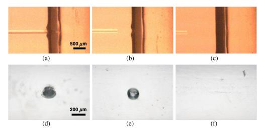
**Fig. 7** TFL with  $100-\mu$ m core fiber placed perpendicular to the silicone catheter wall and operated at 33 mJ and 100 Hz for 1 s. Side view (top) and normal incident view (bottom) after laser exposure at different fiber to wall working distances of (a, d) 0 mm, (b, e) 0.5 mm, and (c, f) 1 mm. These three working distances of 0, 0.5, and 1 mm produced holes, shallow craters, and swelling, respectively.
