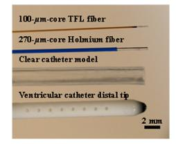
**Fig. 1** Physical dimensions of experimental 100- $\mu$ m core (170- $\mu$ m OD) TFL fiber, standard 270- $\mu$ m core (450- $\mu$ m OD) holmium fiber, clear silicone tubing (1.3-mm ID/2.3-mm OD) catheter model, and distal tip of commercial ventricular catheter (1.2-mm ID/2.2-mm OD).
