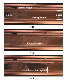
**Fig. 4** Tissue ablation trial showing (a) before laser exposure, (b) after TFL exposure at 50 Hz for 10 s, and (c) after saline irrigation of dislodged debris. An average ablation depth measurement was then obtained for the trial.
