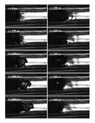
**Fig. 6** High-speed camera images of TFL-induced vapor bubble expansion and collapse during a single 500- $\mu$ s-long laser pulse. The TFL 100- $\mu$ m core fiber was in contact with the tissue phantom in the catheter model. The proximal end of the catheter was open inside the saline container.
