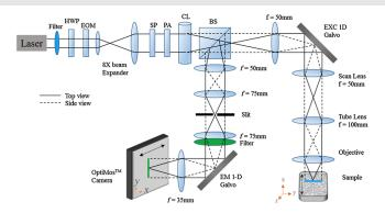
Fig. 1 System schematic. HWP, half-wave plate; EOM, electro-optic modulator; SP, spatial polarizer; PA, polarizing analyzer; CL, cylindrical lens; BS, beam splitter; EXC/EM 1D galvo, excitation/emission 1-D galvo mirrors.
