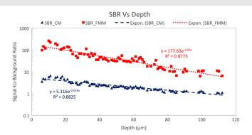
Fig. 3 Plots of SBR for LSFMM (red squares) and LSCM (blue triangles) as functions of imaging depth.
