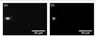
Fig. 2 (a) LSCM and (b) LSFMM images, in the XZ plane, of a fluorescent bead 2  $\mu$ m in diameter.
