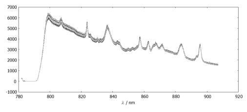
Fig. 7 Raw spectra of an epoxy phantom measured with a single-channel spectrometer at different positions within a square of 2-cm border length.
