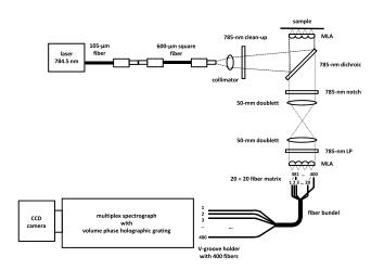
Fig. 1 Setup for generating Raman images from 1-cm<sup>2</sup> skin patches without scanning. See explanation in the text.
