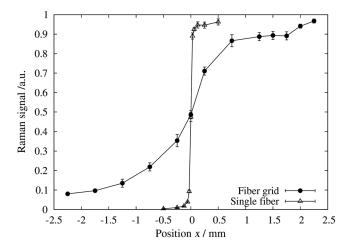
**Fig. 5** Calculated Raman signal (normalized to maximum value) for a large-area Raman source restricted to x > 0 for illuminating all pixels (fiber grid) and a stepwise illumination of only one pixel (single fiber). The abscissa is the position of the receiving fiber relative to the boundary of the Raman source.
