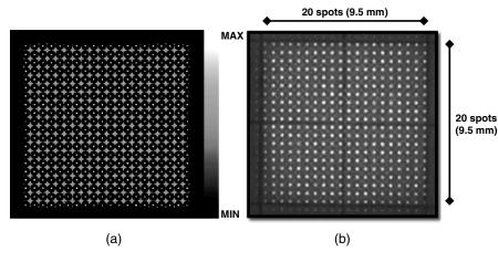
**Fig. 3** (a) Simulated excitation intensity distribution at the sample side. The gray scale is logarithmic. (b) unprocessed (linear) camera image of a scale paper placed on the top of the image acquisition head. The spots show the excitation laser light.
