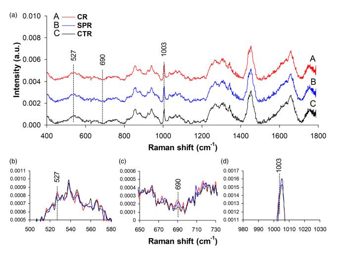
**Fig. 3** (a) Mean Raman spectra of the skin from volunteers with the applied repellent products in spray (SPR) and cream (CR) and the skin without repellent (CTR). Plots of the peaks at (b) 527 cm<sup>-1</sup>, (c) 690 cm<sup>-1</sup>, and (d) 1003 cm<sup>-1</sup> to allow the observation of the overlap of DEET peaks on SPR and CR with the peaks of skin from controls (CTR).
