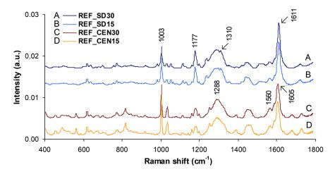
Fig. 5 Raman spectra of sunscreen products of the two bands CEN and SD in two different SPFs (SPF 15 and 30). The labeled peaks represent the most significative peaks.
