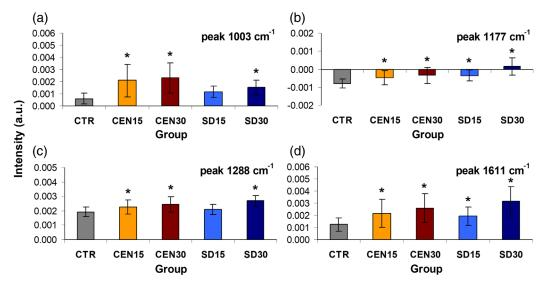
**Fig. 7** Plot of the mean intensity and standard deviation of the Raman peaks of the active ingredients of the sunscreen products found in the spectra of the skin: (a) peak 1003 cm<sup>-1</sup>, (b) peak 1177 cm<sup>-1</sup>, (c) peak 1288 cm<sup>-1</sup>, and (d) peak 1611 cm<sup>-1</sup>. The symbol "\*" indicates a statistically significant difference between the groups CEN15, CEN30, SD15, and SD30 versus CTR when indicated (p < 0.05, ANOVA, and Tukey *post hoc* tests).
