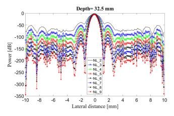
Fig. 8 Lateral variations of NL\_2, NL\_3, NL\_4, NL\_5, NL\_6, NL\_7, NL\_8, and NL\_9 at the depths of 32.5 mm using the images shown in Fig. 7.
