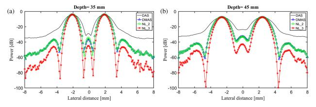
Fig. 4 Lateral variations of DAS, DMAS, NL\_2, and NL\_3 at the depths of (a) 35 mm and (b) 45 mm using the images shown in Fig. 3.
