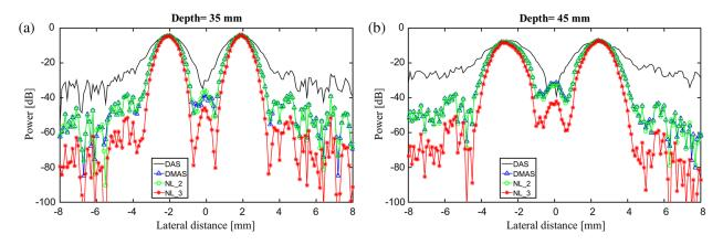
Fig. 6 Lateral variations of DAS, DMAS, NL\_2, and NL\_3 at the depths of (a) 35 mm and (b) 45 mm using the images shown in Fig. 5.
