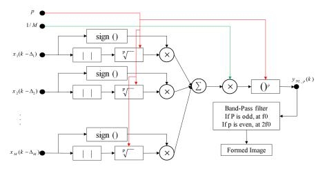
Fig. 1 The flowchart of the proposed NL beamformer.
