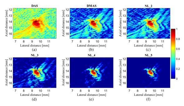
Fig. 10 A zoomed version of the Fig. 9 for better comparison. (a) DAS, (b) DMAS, (c) NL\_2, (d) NL\_3, (e) NL\_4, and (f) NL\_5.
