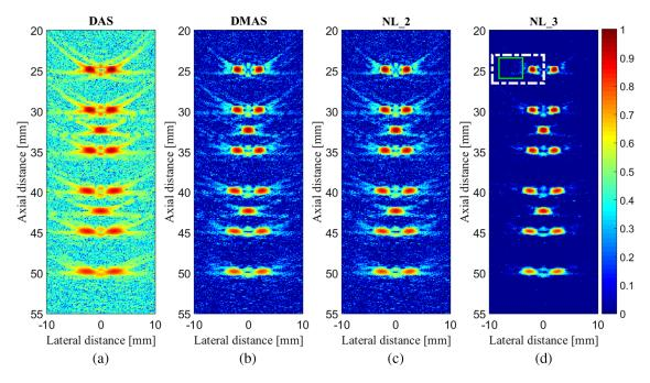
Fig. 5 Images of the simulated point-target phantom. (a) DAS, (b) DMAS, (c) NL\_2, and (d) NL\_3. All the images are shown with a dynamic range of 60 dB. Noise was added to the detected signals considering a SNR of 0 dB.
