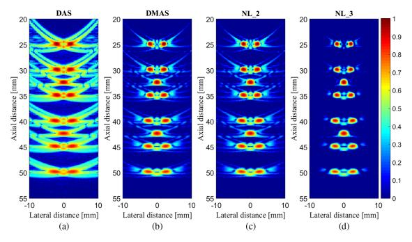
Fig. 3 Images of the simulated point-target phantom. (a) DAS, (b) DMAS, (c) NL\_2, and (d) NL\_3. All the images are shown with a dynamic range of 60 dB. Noise was added to the detected signals considering a SNR of 30 dB.
