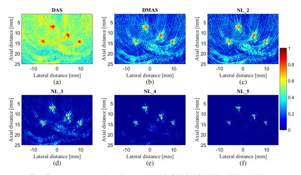
Fig. 9 The reconstructed experimental images using (a) DAS, (b) DMAS, (c) NL\_2, (d) NL\_3, (e) NL\_4, and (f) NL\_5. A wire-target phantom was utilized. All the images are shown with a dynamic range of 70 dB.
