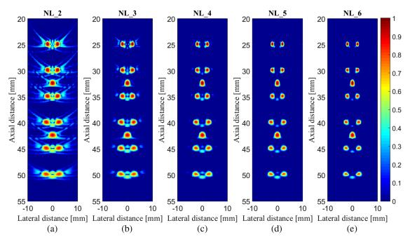
**Fig. 7** Images of the simulated point-target phantom. (a) NL\_2, (b) NL\_3, (c) NL\_4, (d) NL\_5, and (e) NL\_6. All the images are shown with a dynamic range of 60 dB. Noise was added to the detected signals considering an SNR of 30 dB.
