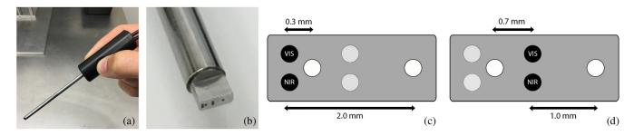
**Fig. 1** (a) The handheld probe of the DRS system used, with a (b) close up of the tip of the probe. (c) and (d) Two different fiber configurations are used to obtain the diffuse reflectance spectra from four different distances between source and detection fibers.
