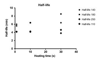
**Fig. 7** The plot shows the half-life obtained from fitting the HIL signal decay using Eq. (1). Except for two outliers, the range of the half-life is between 4 and 7 min. The heating was obtained with a welding device.
