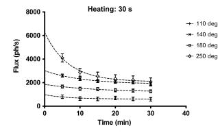
**Fig. 6** The plot shows the decay of the HIL signal and the corresponding fitting (dotted line) for the different temperatures and a heating time equal to 30 s. The heating was obtained with a welding device.
