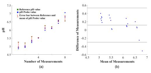
**Fig. 6** (a) *In vitro* measurements: reference measurements using the conventional pH meter in green square, repeatable measurements using the FL system in blue circles, and error bars between average of the three repeated measurements and reference system in red. (b) Bland–Altman plot between reference pH meter and predicted pH values for *in-vitro* tooth samples (using 95% agreement between variables).
