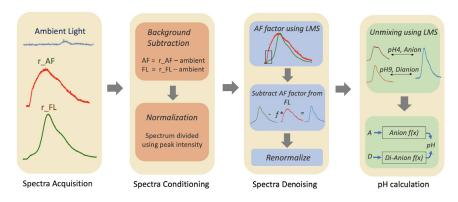
Fig. 3 Procedure for plaque pH measurement.
