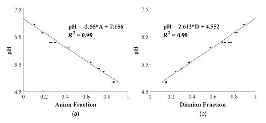
**Fig. 4** Calibration curves obtained using  $200-\mu M$  buffered FL solution in 1-mm glass cuvette. (a) Anion calibration curve and (b) dianion calibration curve.
