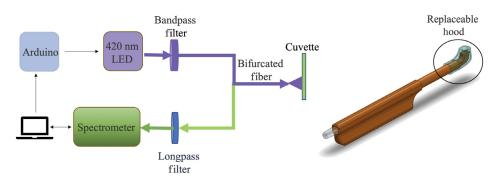
Fig. 1 (a) Diagram of electro-optical device and (b) dental probe.
