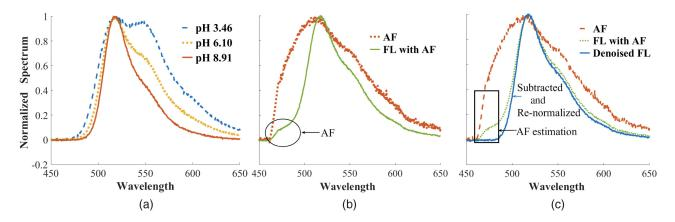
**Fig. 2** (a) FL emission spectrum (450 to 650 nm) for different pH solutions. (b) Tooth AF using 420-nm LED and FL spectrum with noisy AF (c) AF removal. All signals have been normalized using the peak intensity recorded.
