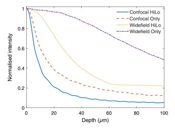
Fig. 5 Optical sectioning performance at different configurations. Normalized intensities are plotted as a function of the depth movement to show axial sectioning profiles at widefield (purple), widefield HiLo (yellow), confocal (red), and confocal HiLo (blue).
