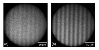
Fig. 3 Grid illuminated images of the fluorescence reference slide at (a) widefield detection and (b) confocal detection.
