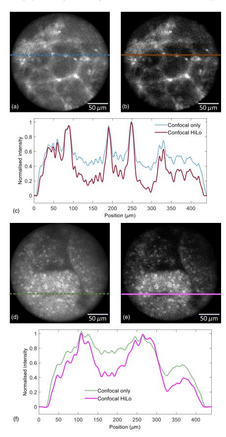
**Fig. 6** Endomicroscopy imaging of porcine kidney tissue. The slit width is set to 6  $\mu$ m in both cases for confocal detection. Perirenal fat (a) without and (b) with the use of HiLo. (c) Intensity plot along the lines indicated in (a) and (b) (blue line: confocal without HiLo and red line: confocal with HiLo). Renal cortex (d) without and (e) with the use of HiLo. (f) Intensity plot along the lines indicated in (d) and (e).
