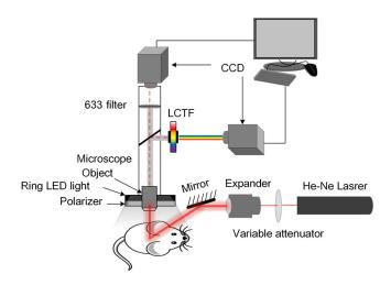
Fig. 1 Schematic of the imaging system.
