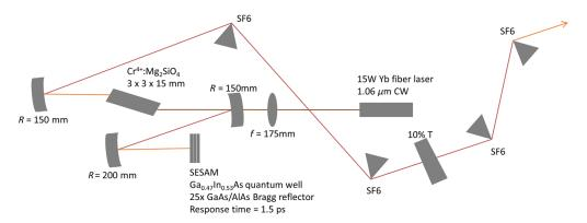
Fig. 2 Schematic illustration of the Cr:F laser oscillator.
