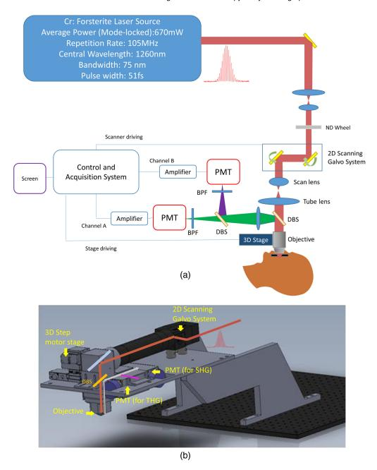
**Fig. 1** (a) A schematic diagram showing the system setup of the HGM used in the clinical trial. (b) The 3-D model of the HGM system. The optical path and important devices are shown. DBS, dichroic beam splitter; BPF, band-pass filter; PMT, phtotomultiplier tube; SHG, second-harmonic generation; THG, third-harmonic generation.
