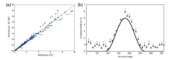
**Fig. 2** (a) Calibration data for an individual  $2\pi$  sr irradiance sensor. Data are shown for two calibrations performed on separate days. (b) Averaged azimuth response of three black backside sensors indicating strong preferential detection from one hemisphere. The solid black line represents a  $\cos(\alpha)^2$  responsivity, here only as illustration.
