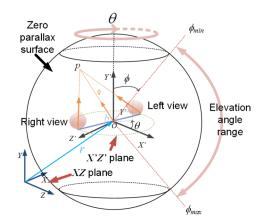
Fig. 1 Binocular viewing model for omnistereoscopic image acquisition where the region of zero parallax (eyes convergence points) is limited to a spherical section, topologically equivalent to a cylinder.
