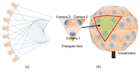
**Fig. 20** Examples of omnistereoscopic cameras based on multiple sensors: (a) in an early patent from 1965, Clay exploited the overlapping FOVs between cameras with slightly different viewpoints to produce stereopsis.<sup>13</sup> (b) Shimada and Tanahashi's multiple-camera configuration designed to produce omnidirectional depth maps in real time.<sup>88,89</sup>
