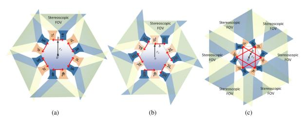
**Fig. 21** Multicamera examples: (a) panoramic camera configuration using multiple stereoscopic pairs in a hexagonal pattern (Baker et al.<sup>93</sup>), (b) different configurations using narrower FOV lenses and larger number of cameras, and (c) an alternative multicamera configuration proposed by the authors.<sup>12</sup>
