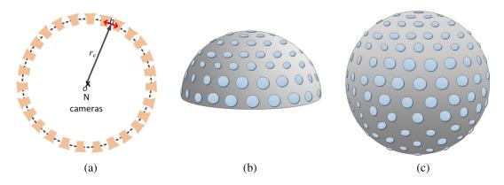
Fig. 22 Multicamera configurations: (a) the camera configuration proposed by Tazvidas et al.<sup>57</sup> in 2002, (b) the omnistereoscopic camera concept developed at the École Polytechnique Fédérale de Lausanne,<sup>97,98</sup> and (c) spherical configuration proposed by Pierce et al. in a patent application.<sup>99</sup>
