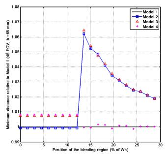
**Fig. 4** The acquisition models are contrasted against the central stereoscopic rig (model 1) showing the relative variation of the minimum distance to the scene to achieve horizontal disparity continuity among neighbor images: the compared configurations are lateral stereoscopic rig (model 2), the lateral-radial stereoscopic rig for  $r_c = b$  (model 3), and the off-centered stereoscopic rig for  $r_c = b$  (model 4).
