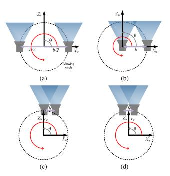
Fig. 3 Omnistereoscopic acquisition models using multiple-camera configurations: (a) central stereoscopic rig, (b) lateral stereoscopic rig, (c) lateral-radial stereoscopic rig, and (d) off-centered stereoscopic rig.
