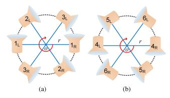
**Fig. 14** Method based on rotating a single camera to capture six stereoscopic images by positioning the camera in 12 different locations and orientations: (a) first, the stereoscopic pairs  $[(1_L, 1_R), (2_L, 2_R), (3_L, 3_R)]$  are acquired one-by-one rotating and positioning the camera to the corresponding locations. (b) Finally, the camera is rotated 180 deg around its nodal point and the pairs  $[(4_L, 4_R), (5_L, 5_R), (6_L, 6_R)]$  are sequentially acquired.
