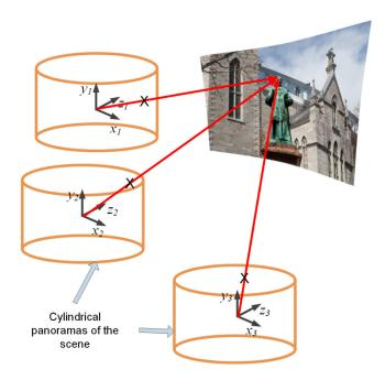
Fig. 16 Multibase stereo reconstruction of a scene based on information acquired from multiple cylindrical panoramas.<sup>82</sup>
