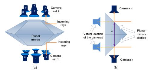
Fig. 9 Omnistereoscopic camera configuration based on coaxial planar mirrors: (a) configuration based on Kawanishi et al.'s idea<sup>27</sup> and (b) virtual location of each camera's projection center and vertical baseline *b*.
