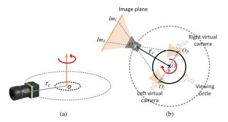
**Fig. 13** Rotating method to produce omnistereoscopic imagery based on a single rotating camera: (a) a single camera is rotated from an offcentered location and (b) two projections corresponding to left- and right-eye projections can be defined intersecting the rays passing through the camera's projection center O and the points  $O_L$  and  $O_R$  defined over a virtual viewing circle.
