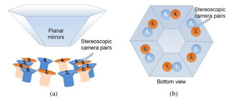
Fig. 10 Omnistereoscopic video camera developed at the Fraunhofer Heinrich-Hertz Institute: (a) each planar mirror face is associated with a stereoscopic pair of cameras, (b) locations the cameras as seen reflected on the planar mirrors.
