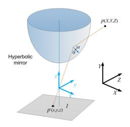
Fig. 6 SVP catadioptric camera principle using parabolic mirrors.
