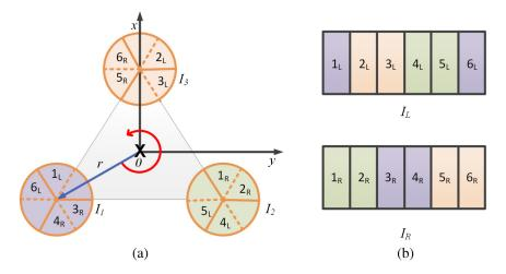
**Fig. 19** Omnistereoscopic images using a cluster of three panoramas: (a) three cylindrical panoramas  $(I_1, I_2, I_3)$  in a coplanar, triangular pattern can be used to extract six image sections, and then mosaicking them using the sequence illustrated in (b) to create two novel stereoscopic views  $(I_L, I_R)$ .
