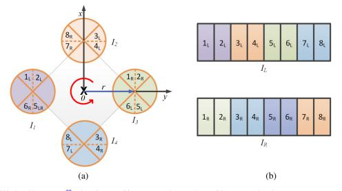
**Fig. 17** Vanijja and Horiguchi proposed<sup>20</sup> using clusters of four panoramic snapshots of the scene taken in a square pattern, to extract eight wideangle stereoscopic images to render a full omnistereoscopic image: (a) the mapping of the eight image sections from panoramas  $(I_1, I_2, I_3, I_4)$  and (b) the mosaicking of these sections to create a cylindrical omnistereoscopic pair  $(I_L, I_R)$ .
