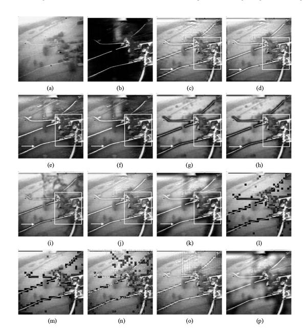
Fig. 14 Fused images of several fusion algorithms and with the nonoverlapping block method. (a) and (b) Navigation source images. (c) DWT. (d) SWT. (e) NSCT. (f) LPSSIM. (g) SR. (h) SOMP. (i) JSR. (j) MODJSR. (k) NSCTSR. (l) SR\_S8. (m) SOMP\_S8. (n) JSR\_S8. (o) MODJSR\_S8. (p) NSCTSR\_S8.
