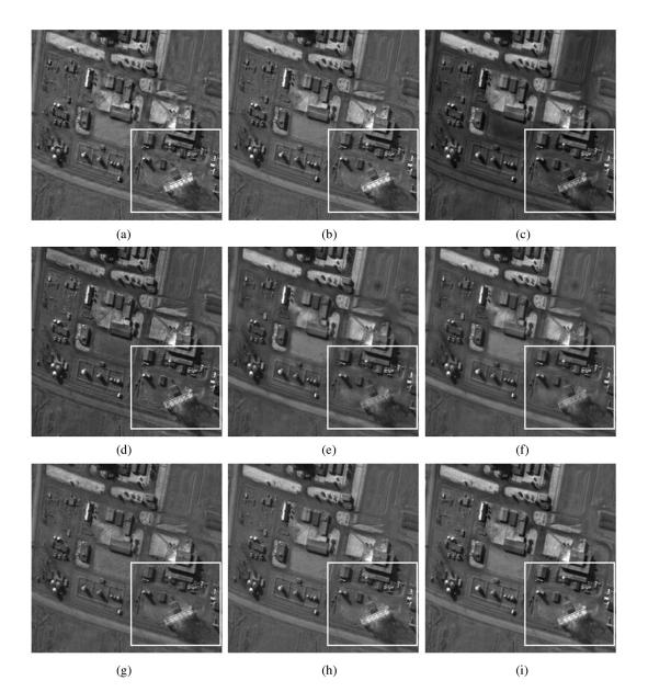
Fig. 10 The "input094" multisensor source image fusion results using (a) DWT, (b) SWT, (c) NSCT, (d) LPSSIM, (e) SR, (f) SOMP, (g) JSR, (h) MODJSR, and (i) NSCTSR.
