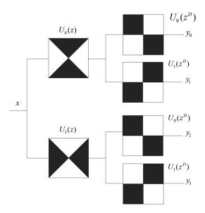
Fig. 3 Four-channel nonsubsampled filter bank constructed with two-channel fan filter banks.
