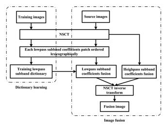
Fig. 5 Procedure of image fusion based NSCT and sparse representation.
